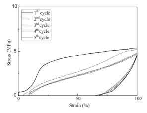
**Figure 2.**Thermomechanical cyclic tensile testing curves of the PUHCO2-5 polyurethane.
