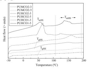
**Figure 1.**DSC thermograms of synthesized polyurethanes.
